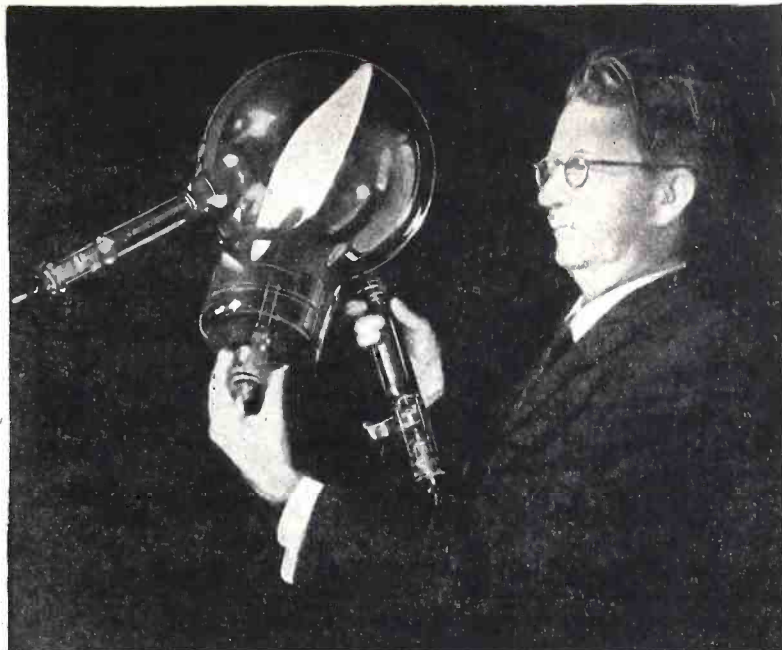
Mr. J. L. Baird with his recently invented color-television tube.
